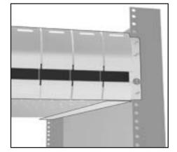
5. Snap the end cap over the screw on each side of the unit to finish the installation.
